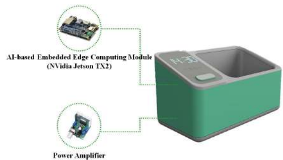
FIGURE 4. Structure of the proposed AI-based intelligent drug pill recognition box.
