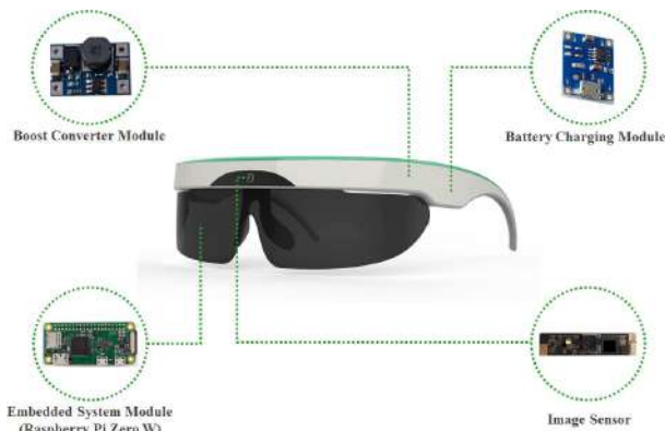
FIGURE 3. Structure of the proposed wearable smart glasses.
