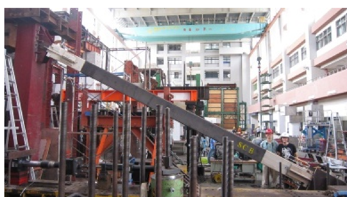
Fig. 2. 8 m-Long Dual-Core SCB Test to 2% Drift (Maximum Peak Force 1700 kN)
