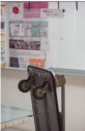
Residual-glue-free adhesives designed to fix heavy weights of objects (e.g. cart)
