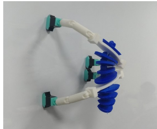
Residual-glue-free adhesives for climbing robot's movement
